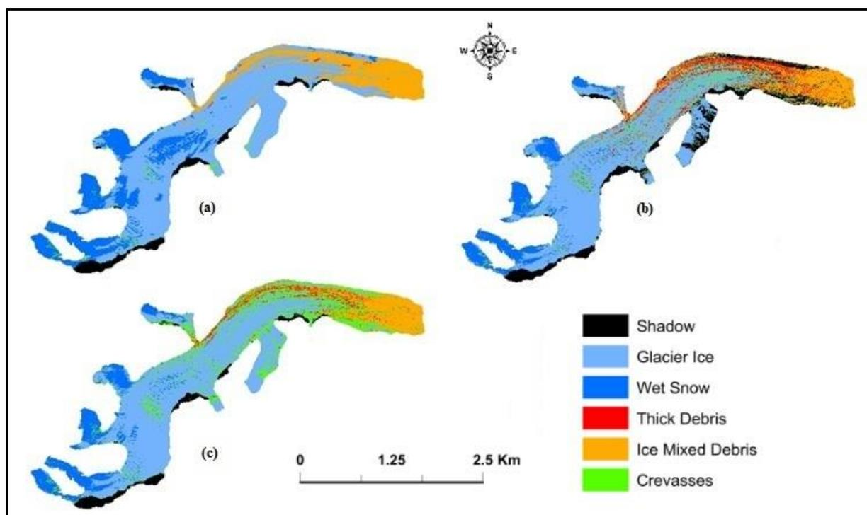
Figure 4. (a) Facies classification using OOC method, (b) Facies classification using MH method, (c) Facies classification using MXL method.
