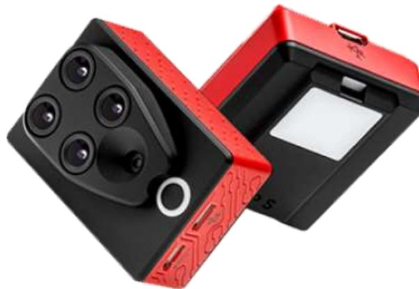
Figure 4: Parrot Sequoia Multispectral sensor and Sunshine Sensor
