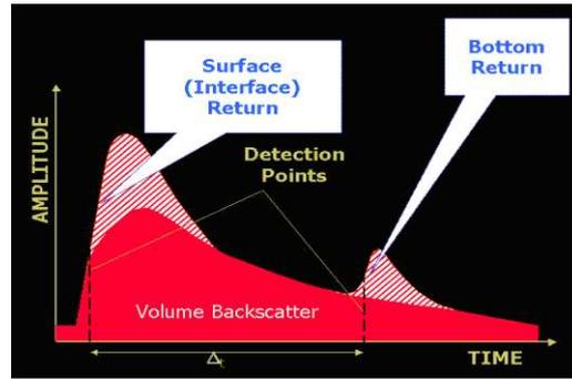
Figure 1: Generic received lidar signal (Guenther *et al.*, 2000).
