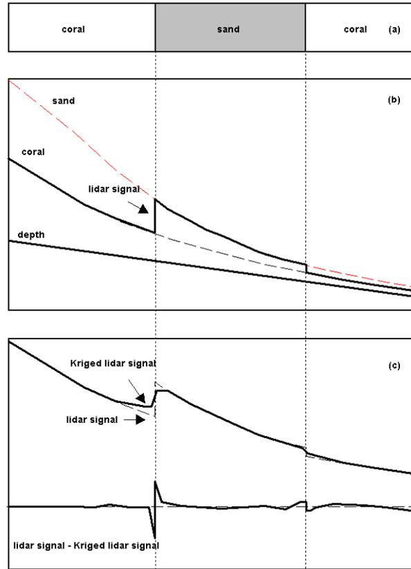
Figure 2: Using kriging technique to detect ocean bottom change. Panel (a) shows a imaginary site consist of two bottom types, sand and coral. Panel (b) shows the depth profile of this site, the therotical lidar signal of sand and coral at different depth, and the lidar signal of this imagernary site. Panel (c) shows the lidar signal after being smoothed by kriging, and the difference between the original lidar signal and the smoothed lidar signal.
